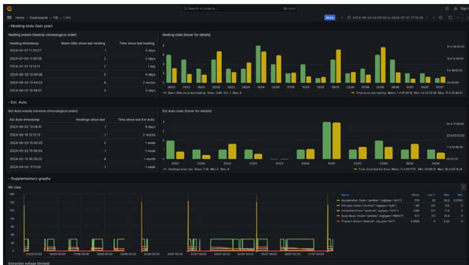
Figure 1: Long-term performance statistics on ion source performance, an important health metric for advanced focused ion beam instruments.
